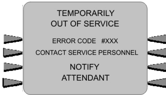
Figure 7-23. Initial "Out of Service" screen
